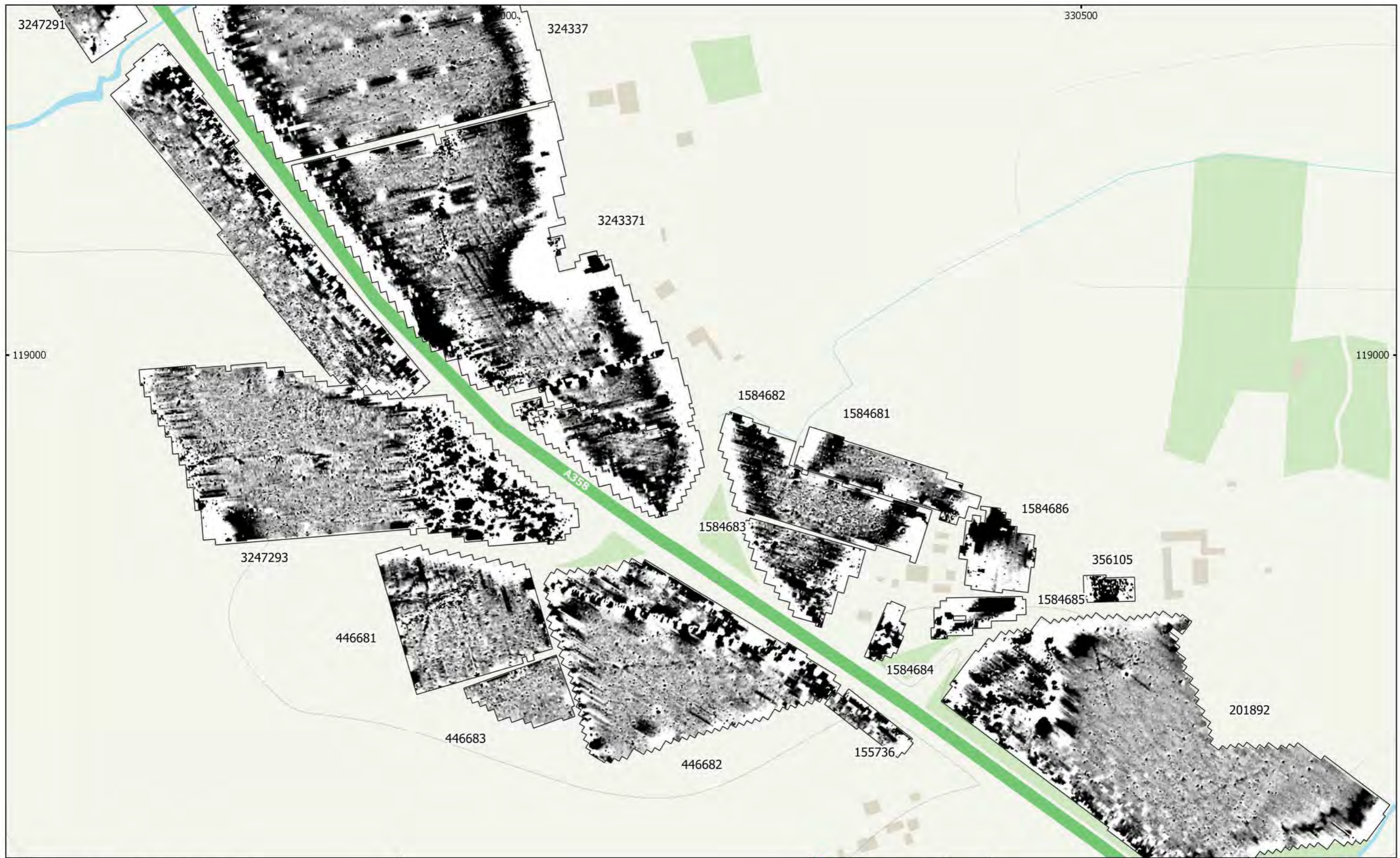
MSST901 - A358 Taunton to Southfields Dualling Figure 24 - Magnetic Total Field (Lower Sensor) (Overview 10 of Zones 2 & 3) 1:3,000 @ A3 Copyright Magnitude Surveys Ltd 2021 Contains Ordnance Survey data © Crown Copyright and database right 2021
